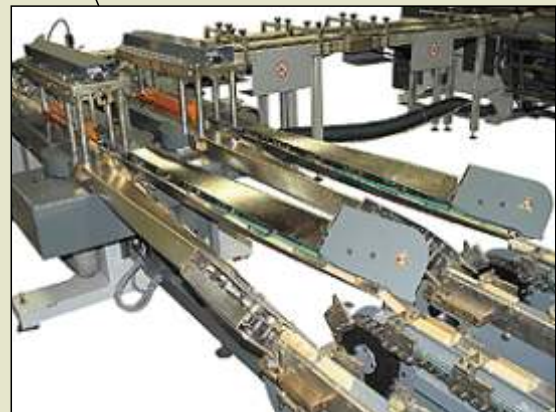
SMA 112 Chains of 1 inch for the transport of the triangles.
