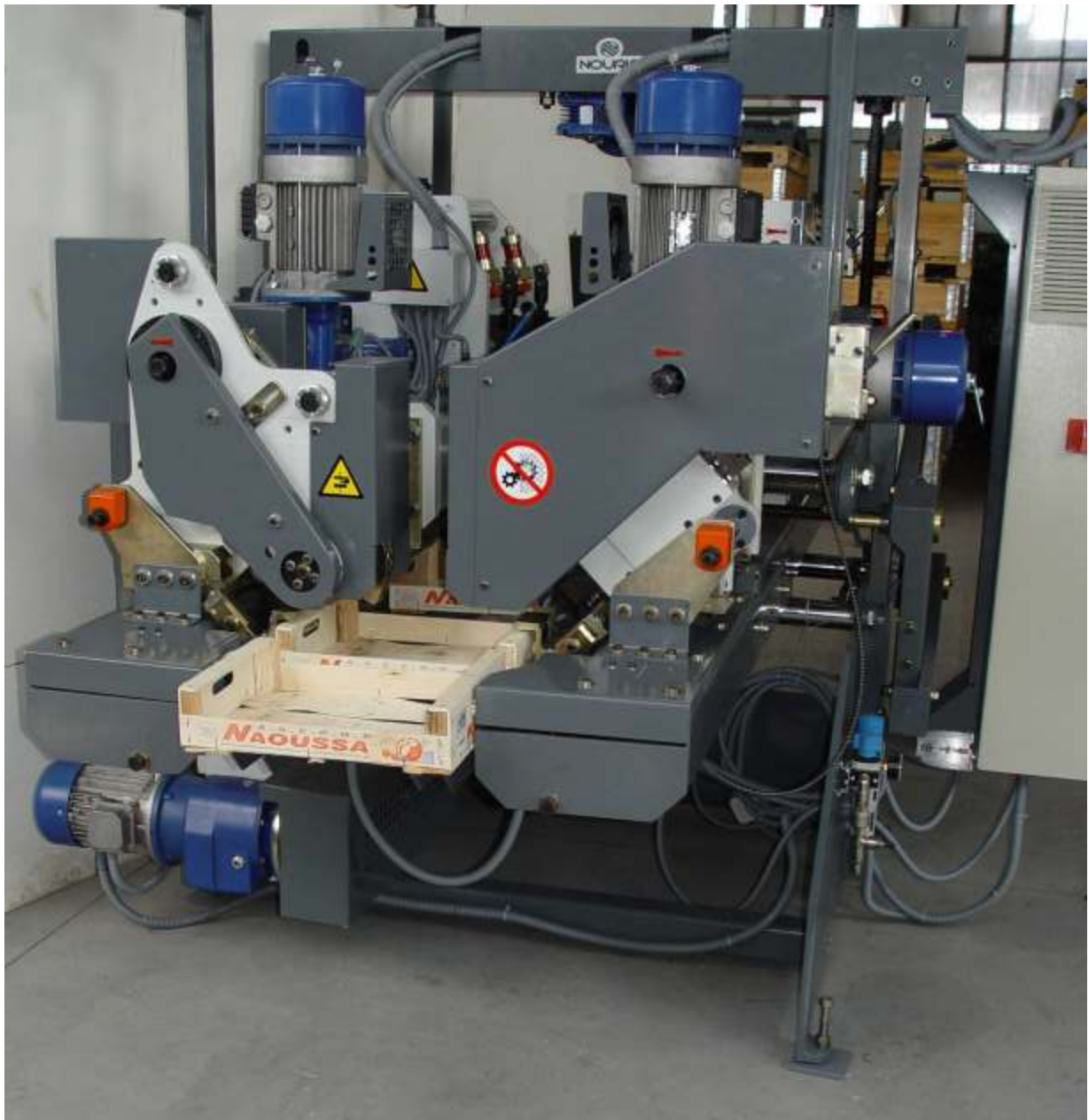
TYPE SMA121C: Two angle stitching heads at the exit type monoblock for the stitching at the middle of the barret.
