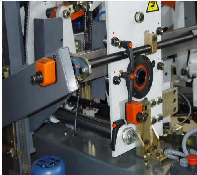
Four stitching heads with monoblock system. Easy, fast and accurate adjustment.
